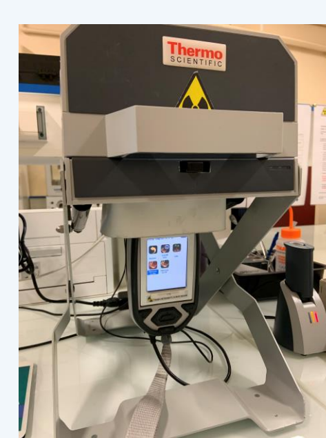
XRF Portable Niton XL3t Gold++
